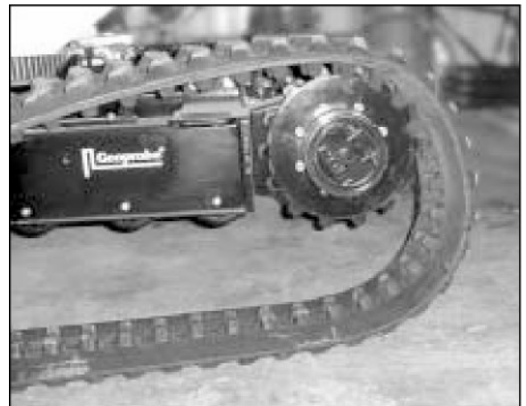
Figure 9: Place the rubber track over the drive wheel sprocket.
