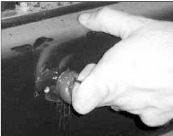
Figure 7: Grease will escape from the tube as the tension wheel is retracted to loosen the track.
